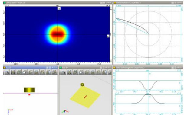
Result for a gap of 0.1mm and the sensor oriented perfectly parallel to the plate. C-scan image, impedance plane, channel X (real) and channel Y (imaginary).
