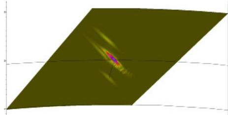
Same crack tilted 30° - height of 4 mm
