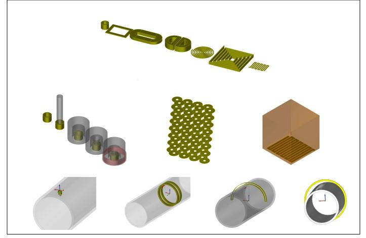
Various ET probe configurations in CIVA: Numerous shapes of coil available, rotating probe or bobbin coil in tubes, bobbin coils, encircling coil, sectorial coil, EMAT probe, Eddy Current Arrays
