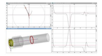
Inspection of a tube transition zone in a tube exchanger
