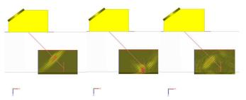
Snapshots of the beam/flaw interaction vs time
