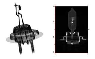
Once the processing is finished, a new analysis page opens with the 3D reconstructed specimen. The 3D view available in CIVA shows the component in 3D dimensions. Many tools are then available to represent the reconstructed component: Display of the **iso surfaces**, **volume rendering**, etc.
