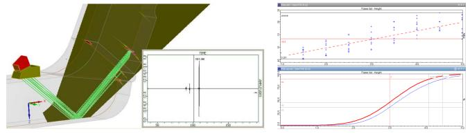
Inspection simulation results: S-Scan, A-Scan, POD curve, etc.
