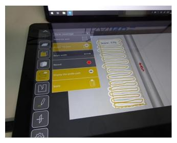
This level of performance accounts for the beam width, that depends on the UT probe used, and also accounts for the probe skew to make sure you scan with a good orientation.
