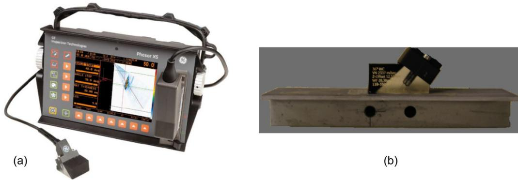
Figure 2.—(a) The General Electric (GE) Phasor XS portable ultrasonic flaw detector. (b) Phased array probe positioned on the external side (top) of the isogrid test part.
