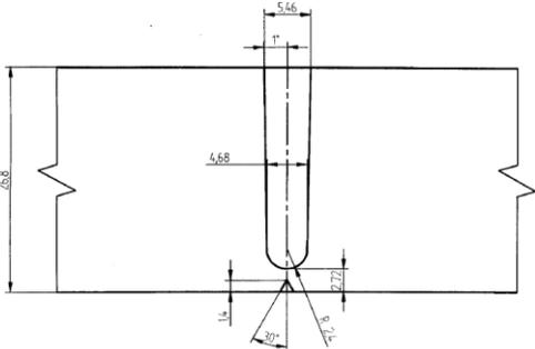
Figure 3: 1° J-Bevel weld cross-section
