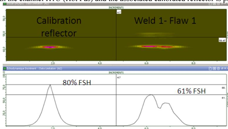
Figure 8: Simulated CIVA D-Scan and echodynamic charts for Weld1-Flaw1 with Channel H1U
