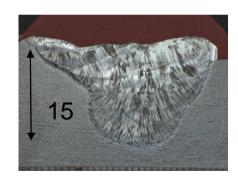
Weld repair – alloy 82 – GTAW
