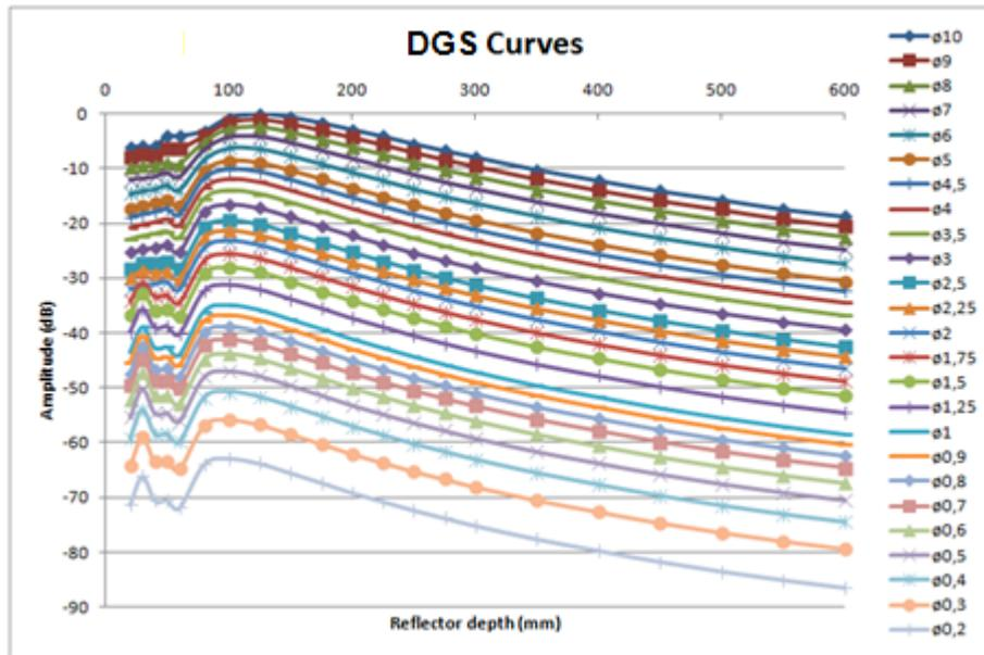
Figure 4. DGS curves computed for several FBH diameters
