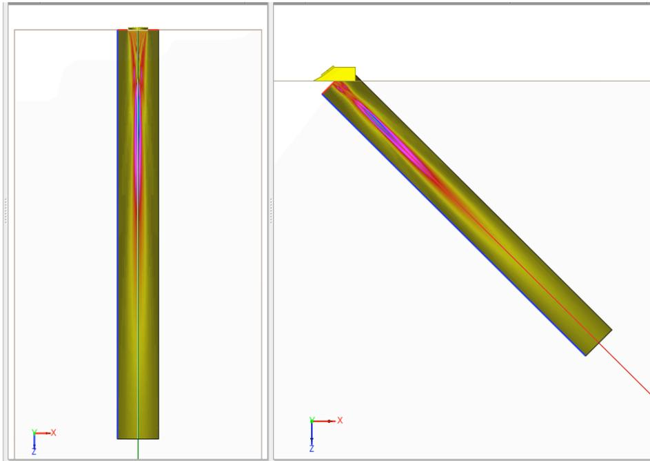
Figure 2. Fields of L0 and T45 transducers, simulated by CIVA
