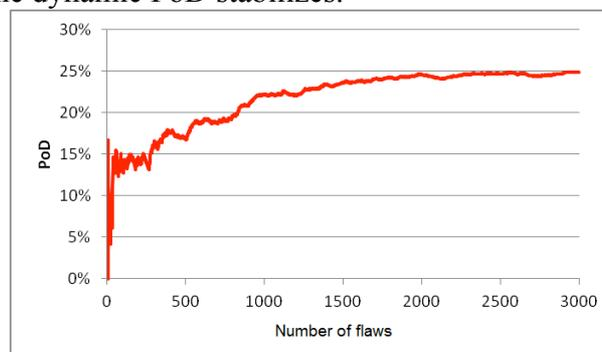
**Figure 6. Dynamic PoD for one probe and for a given safety factor  $f_s$**
