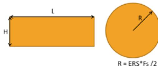
**Figure 1. Detection Criteria, Surface of rectangular flaw and disc of equivalent ultrasonic response**
