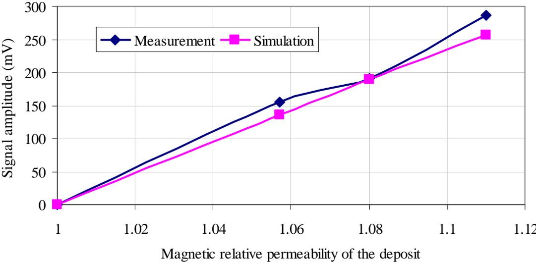
Figure 6 - Effect of the magnetic permeability of the deposit material on the axial probe signal
