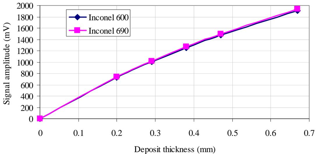
Figure 8 - Influence of tube material on the axial probe signal
