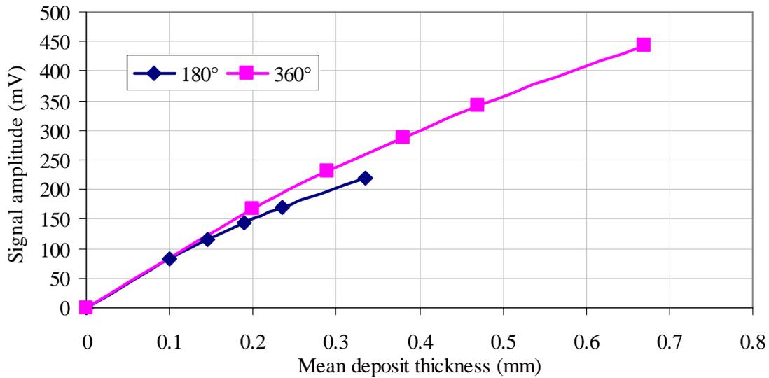
Figure 9 - Deposit geometry effect on the axial probe signal
