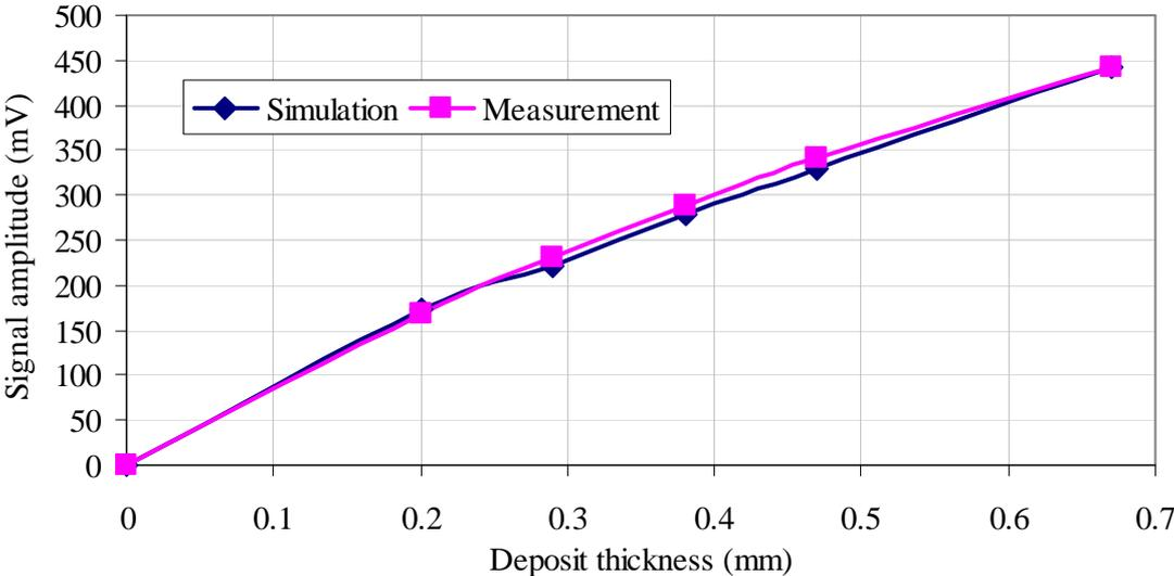
Figure 5 - Effect of the thickness of the deposit on the axial probe signal
