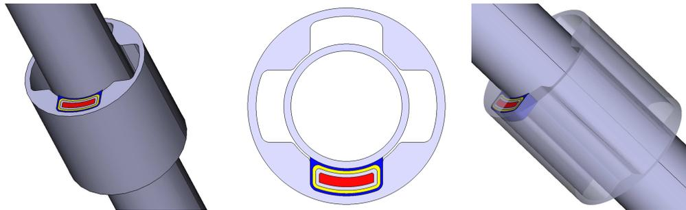
Figure 10 - Clogging configuration of the mock-up numerical models. The tube is centered in the support plate. The plate diameter has been reduced with no effect on the results. Blue, yellow, grey and red clogging volumes correspond to the different clogging occlusion values (blue: 25%, + yellow: 50%, +grey: 75%, +red: 100%). Here clogging is drawn only in one hole but it is present in all four holes.
