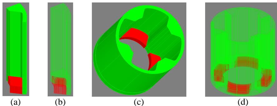
Figure 11 - Flux3D numerical model of the mock-up, in red the clogging volumes, in green the tube support plate. (a) and (b), 1/8<sup>th</sup> of the actual geometry used for the computation, (c) and (d) full geometry when the symmetry conditions are applied
