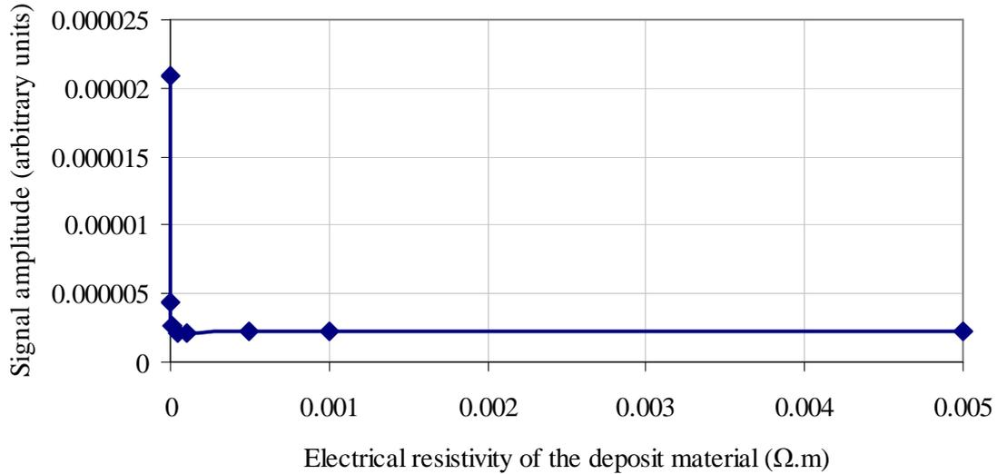
Figure 7 - Influence of electrical resistivity of the deposit material on the axial probe signal ( $\mu_r=1.08$ )
