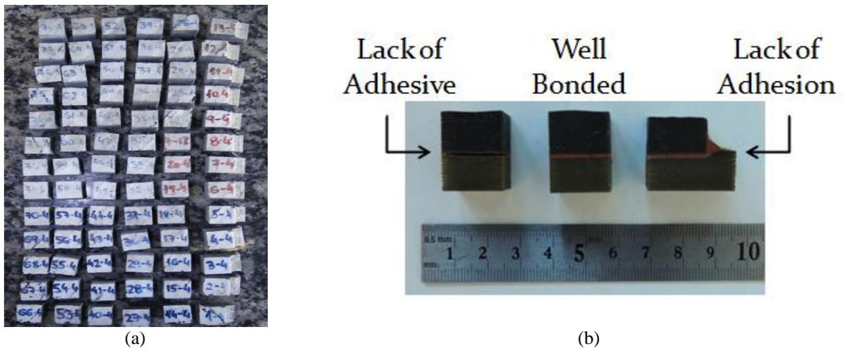
FIGURE 12. Example of one of the specimens after cutting. (a) One whole sectioned joint and (b) examples of some of the obtained sections, presenting the simulated defects.
