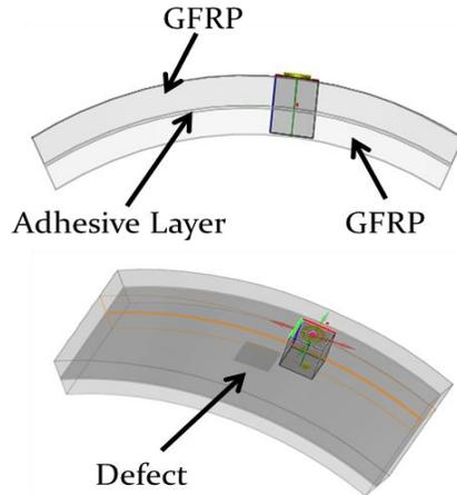
FIGURE 1. 3D CAD specimen applied in CIVA for the performed simulations.
