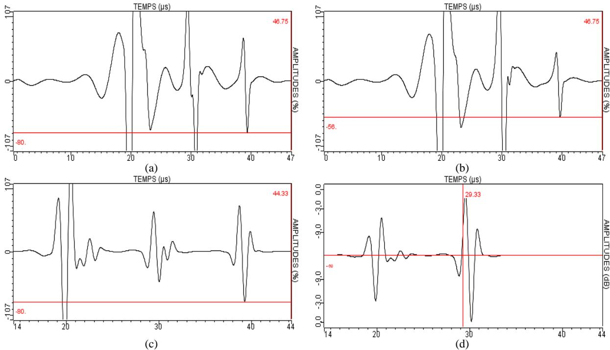
**FIGURE 14.** A-scans produced by CIVA for the 1MHz focused transducer: (a) Signal from a non defective area, (b) Signal from an area with lack of adhesion, with the rise of amplitude of the second echo (adhesive layer echo) and the third echo (backwall echo) attenuated. (c) Signal from a non defective area and (d) signal from an area with lack of adhesive, with the rise of amplitude of the second echo (adhesive layer echo) and the inexistence of the third echo (backwall echo).
