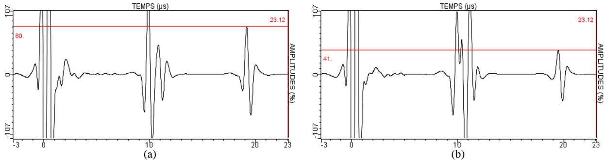
**FIGURE 5.** A-scans produced by CIVA for the frequency of 1.6MHz: (a) Signal from a non defective area and (b) Signal from an area with lack of adhesion, with the rise of amplitude of the second echo (adhesive layer echo) and the third echo (backwall echo) attenuated.
