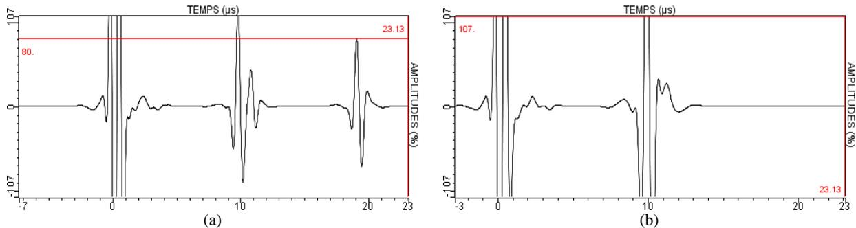
**FIGURE 6.** A-scans produced by CIVA for the frequency of 1.6MHz: (a) Signal from a non defective area and (b) Signal from an area with lack of adhesive, with the rise of amplitude of the second echo (adhesive layer echo) and the inexistence of the third echo (backwall echo).
