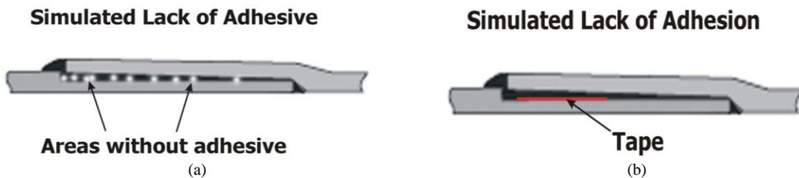
**FIGURE 3.** Studied defects: (a) Lack of Adhesive simulated defect and (b) Lack of Adhesion simulated defect.
