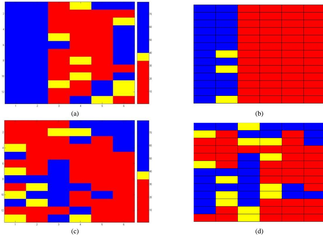
**FIGURE 13.** Comparison between ultrasonic C-scans and the real state of the joints. (a) Ultrasonic C-scan for the sample Lack of Adhesion 4-2, (b) Real state of the sample Lack of Adhesion 4-2, (c) Ultrasonic C-scan for the sample Lack of Adhesive 8-2, (d) Real state of the sample Lack of Adhesive 8-2
