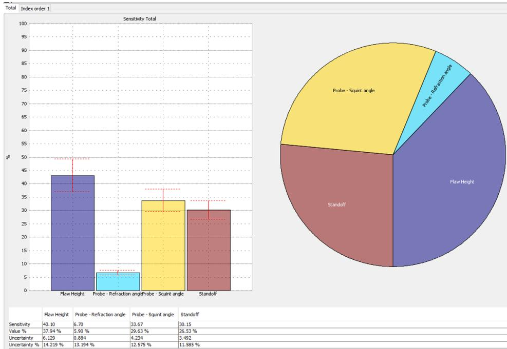
**Figure 9. Sobol Indices ranking influential parameters (flaw height, probe squint and refraction angles, probe standoff) impact on the output signal depending on their variability.**
