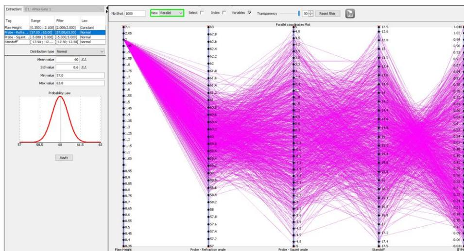
**Figure 8. Parallel plot of 1000 inspection scenarios giving the signal amplitude variability (right column) assuming a constant flaw height of 2mm (1st column), and gaussian variability laws for refraction angle, squint angle and probe standoff (2<sup>nd</sup> to 4<sup>th</sup> column)**
