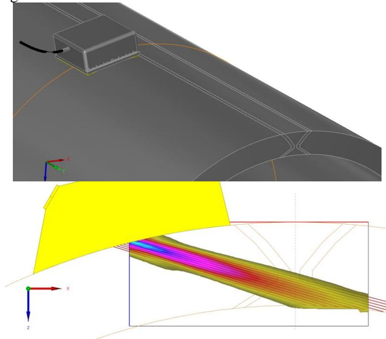
**Figure 2. Model of the AUT system (L7 channel) in CIVA user interface and UT field (above-12dB)**
