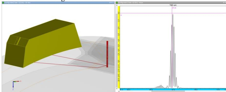
**Figure 3. Response of the calibration reflector (Hole of 1.6mm diameter)**
