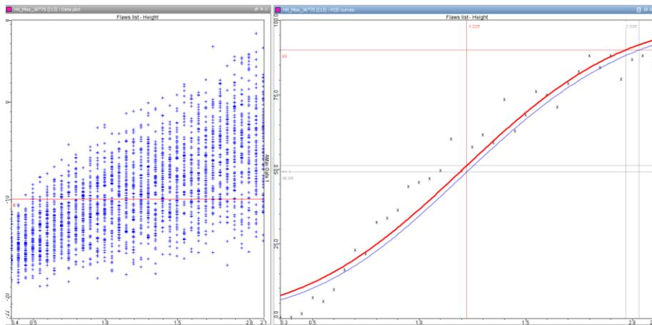
**Figure 11. Data points (on the left) and Hit Miss POD curve based on a metamodel data set of 2700 points.**
