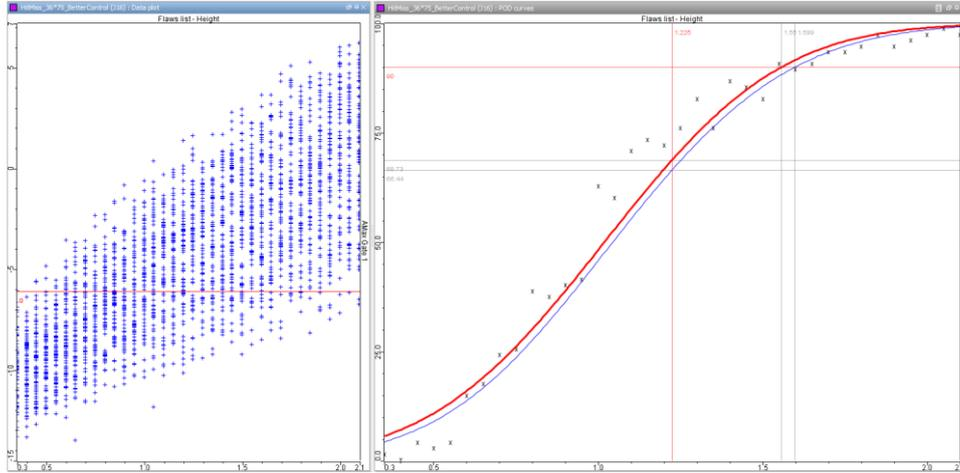
Figure 12. Data points and Hit Miss POD curve with less variability on the inspection parameters.
