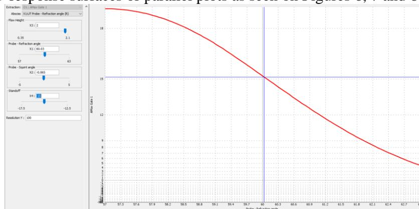
**Figure 6. Impact of a refraction angle variation from 57° to 63° on signal amplitude (in dB calibrated versus TDH) for a flaw height of 2mm, probe squint of -2° and probe standoff of 60mm.**
