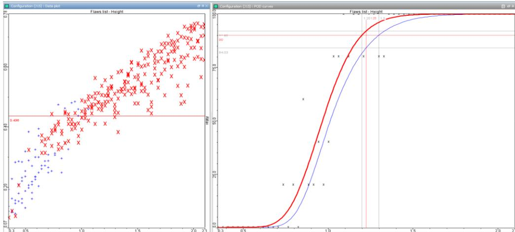
Figure 13. POD curve with L7 and L3 channels response
