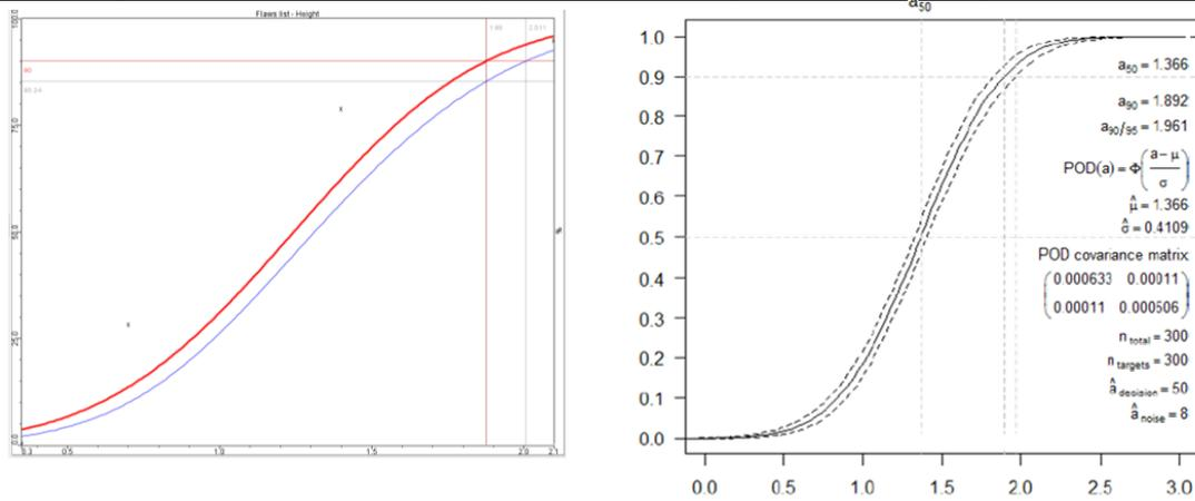
**Figure 10. Signal Response POD curves based on a metamodel data set of 300 points (on the left) and experimental POD curves (on the right).**
