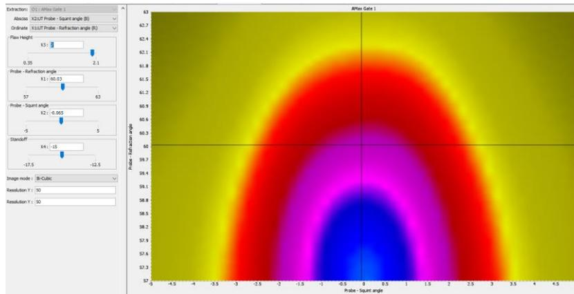
**Figure 7. Impact of a refraction angle variation from 57° to 63° and a squint angle variation from -5° to +5° on the signal amplitude for a flaw height of 2mm and probe standoff of 60mm.**
