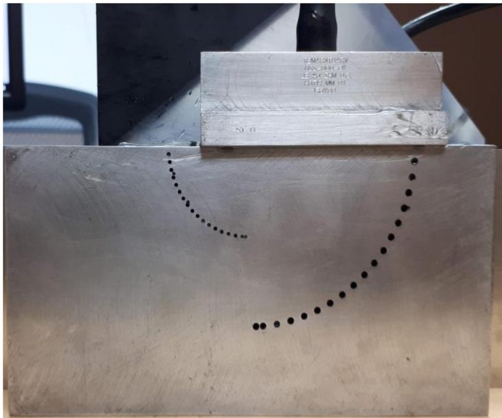
Figure 2. ASTM E2491 PA Assessment Test Block (Type B) with a challenging distribution of side drill holes.
