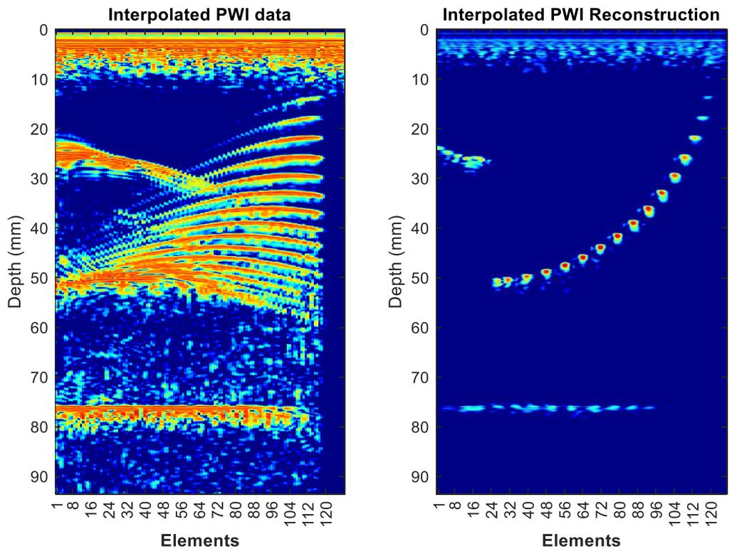
Figure 5. The left plot shows the interpolated PWI data and the right image depicts the reconstructed data from the dense matrix.
