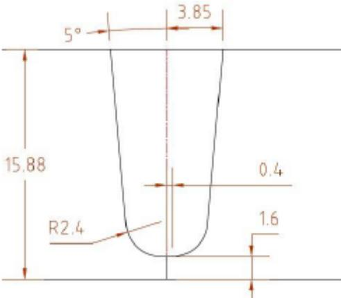
Figure 1 Qualification weld parameters
