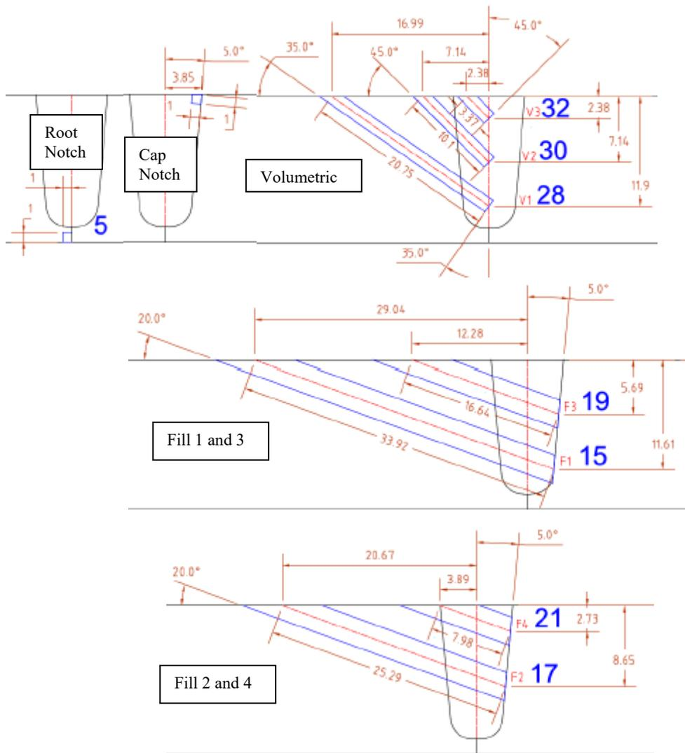
**Figure 2** Field qualification calibration targets
