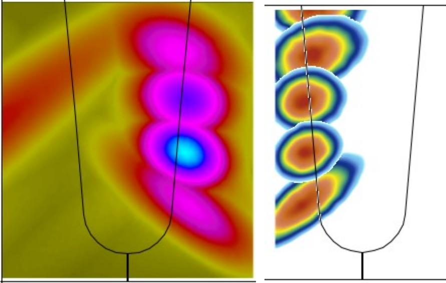
**Figure 7** Sensitivity Coverage in 4 Fill Zones relative to maximum (left). Equalised and indicating to -6dB on overlays (right)
