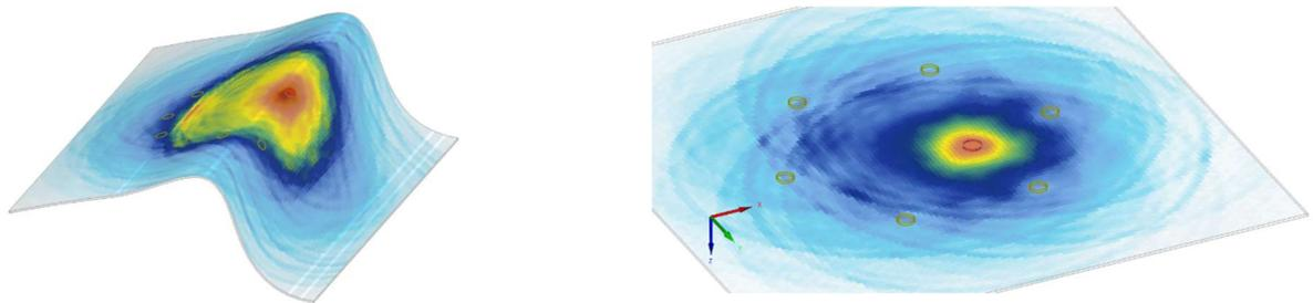
Local fields of displacement and stress can be extracted for further visualizations. CIVA SHM also includes a semi-analytical tool for dispersion curve computation and analysis.
