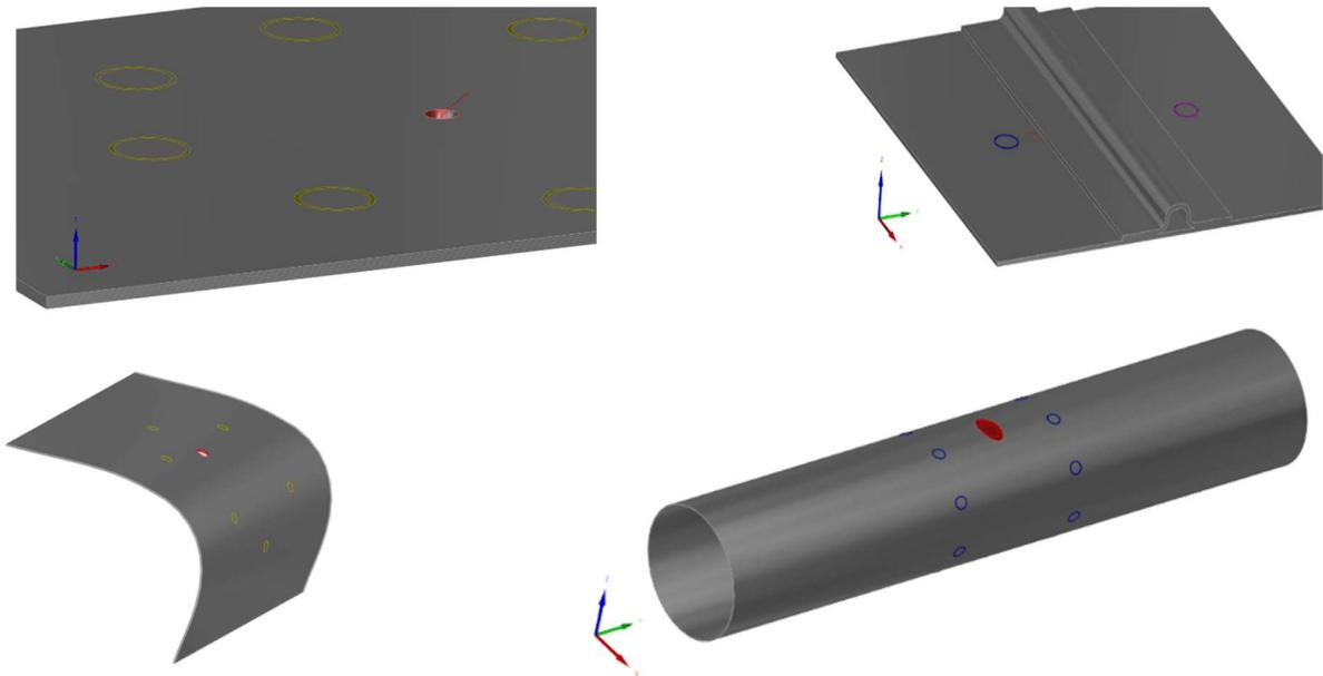
An **array of Guided Wave sensors** can be defined around the defective zone and work in Round Robin or custom scan mode. Radial, normal or custom excitation profiles can be assigned to the sensors. Inspection simulation tools will compute the signals received on each sensor. From these results, an **imaging reconstruction algorithm** (“Delay and Sum”) is available to process these results and give an image of the defect impact displayed on the 3D view for the different wave modes.
