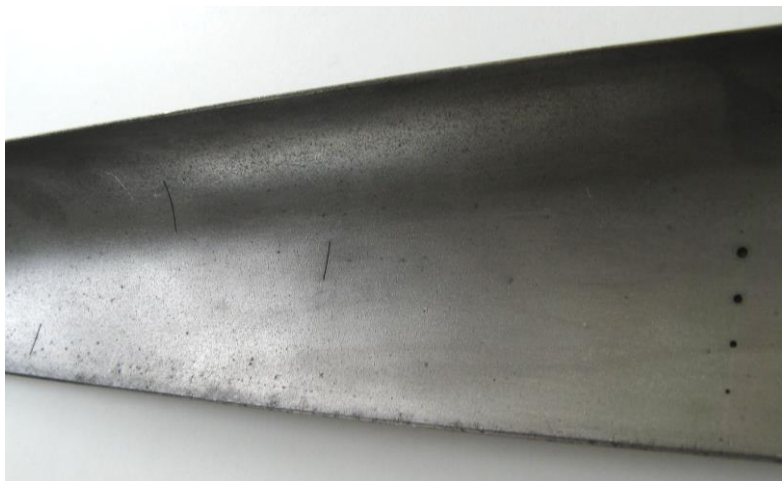
EDM defects - SDH - semi-elliptical groove
