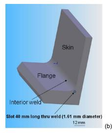
Figure 1.—(a) Actual photograph of interior of Ares USS segment and (b) solid model for the skin-to-flange test sample.
