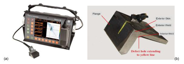
Figure 2.—(a) The General Electric (GE) Phasor XS portable ultrasonic flaw detector and (b) Phased array probe positioned on the external side of the skin of the skin-to-flange test part.
