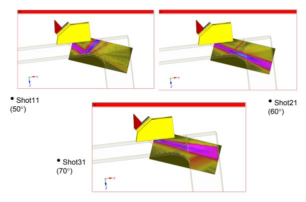
Figure 6.—Beam profile ultrasonic modeling results at several angles in the sectorial scan.
