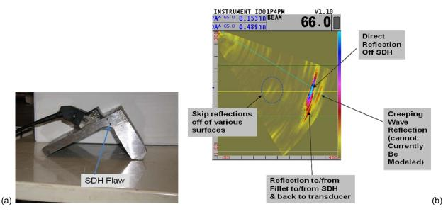
Figure 4.—(a) Probe location for (b) 40° to 75° sector scan results.
