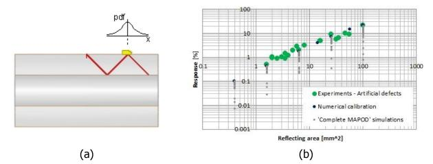
*Figure 7* Application of the "complete MAPOD" approach: a) model definition; b) comparison between 2<sup>nd</sup> leg experiments and numerical results
