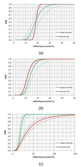
Figure 8 POD curves: calibration; b) transfer function; c) complete MAPOD
