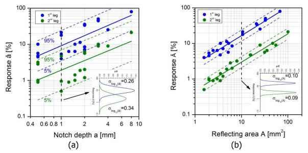
Figure 2 Comparison between UT responses in terms of (a) depth and (b) reflecting area
