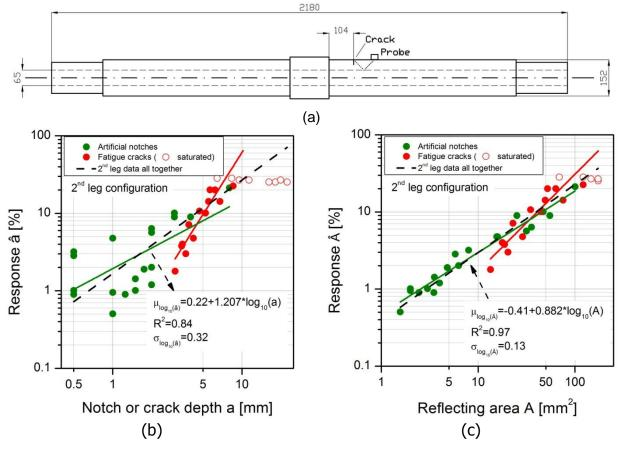
*Figure 3* UT responses of natural fatigue cracks: a) full-scale axle; b) results in terms of depth; c) results in terms of reflecting area
