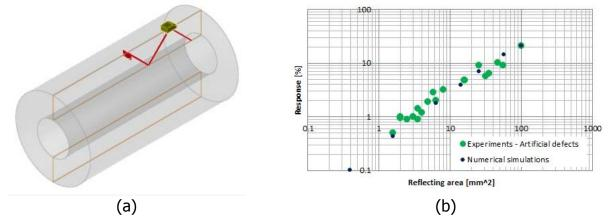
*Figure 5* Calibration of the numerical model: a) numerical set-up; b) comparison between 2<sup>nd</sup> leg experiments and numerical results
