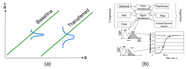
Figure 4 Two MAPOD approaches [8]: a) transfer function; b) complete approach
