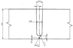
Figure 3: 1° J-Bevel weld cross-section
