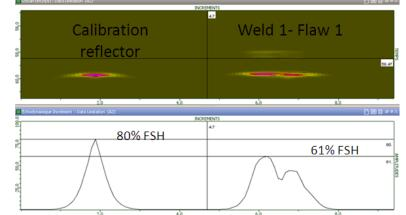
Figure 8: Simulated CIVA D-Scan and echodynamic charts for Weld1-Flaw1 with Channel H1U
