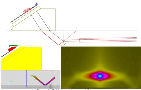
Figure 5: F2U channel views: a) Ray tracing, b) Transmitted beam calculated in the incident plane, c) spot sizing in the weld plane (2.9mm\*4.4mm at -6dB)
