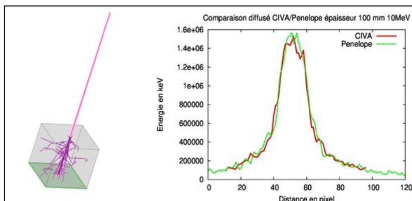
Figure 10: Validation of the scattering effect for high energy in CIVA
