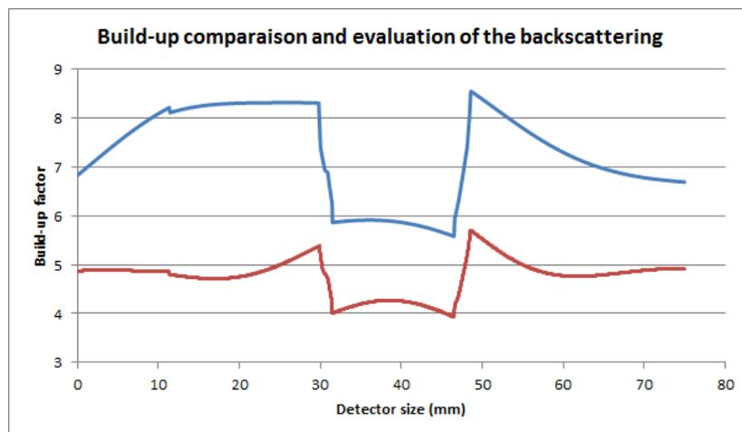
Figure 12: Comparison of the Build-up mapping on the two configurations (Blue curve: Back scattering accounted for, Red Curve: Backscattering ignored)
