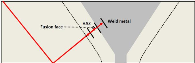
Figure 6: Acquisition gate adapted to fusion line region inspection
