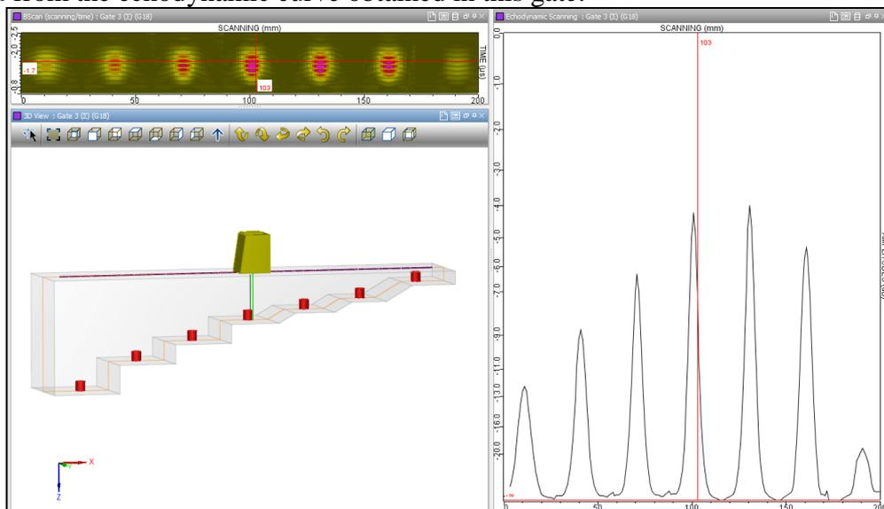
Figure 4: DGS curve obtained thanks to the application of a relevant acquisition gate in a modified step wedge block
