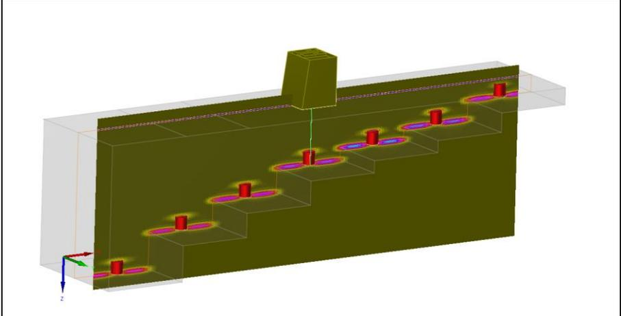
Figure 2: Carbon Steel Step Wedge, Results obtained without applying acquisition gates
