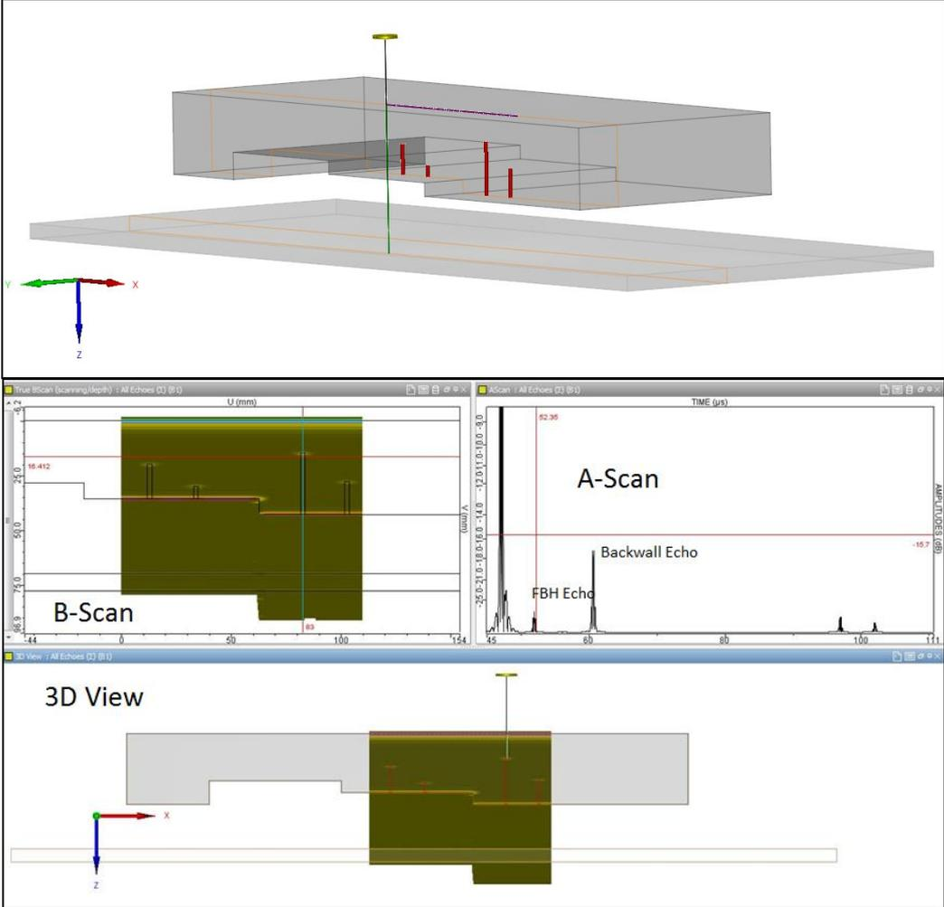
Figure 1: Simulation of a test setup involving several solids (aluminum block and glass plate) and obtained results
