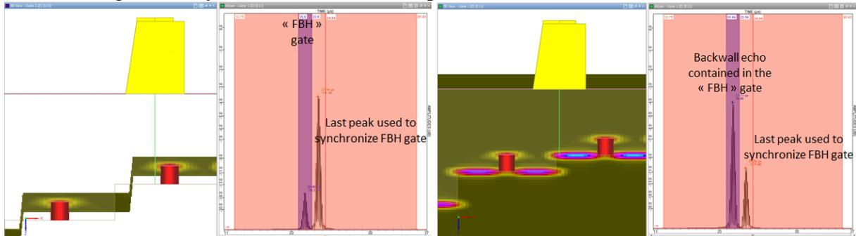
Figure 3: Gate definition versus backwall echo: Left image: FBH echo isolated, Right image: Additional backwall echo “trapped” in the gate
