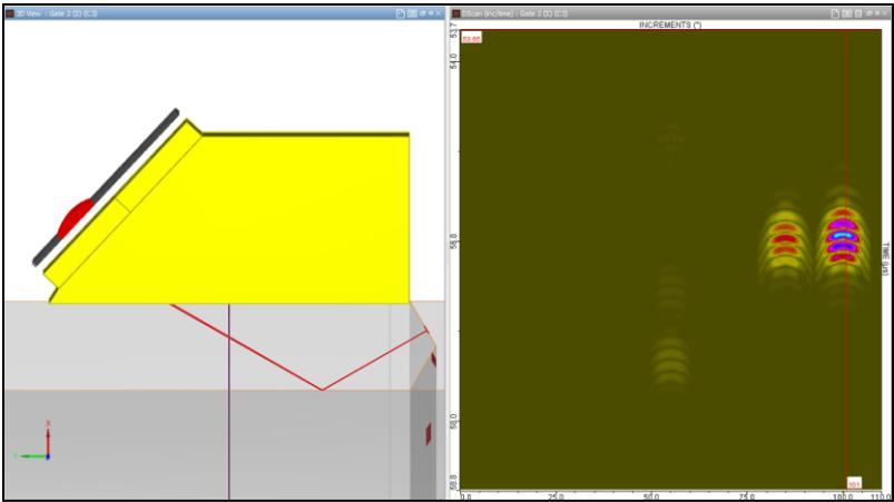
Figure 7: X-Bevel AUT inspection – B-Scan obtained with one channel (Lack Of Fusion echo) –
