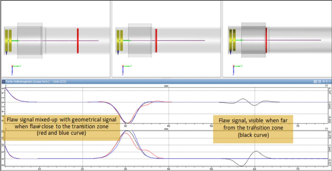
Figure 8: Tube transition zone inspected with a 200 kHz bobbin differential coil, axisymmetric flaw respectively located at 25 mm (black curve), 5mm (red curve) and 1mm (blue curve) from the starting of the tube transition zone
