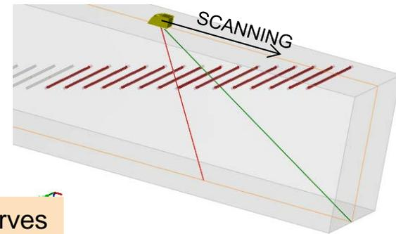
Contact  $\varnothing 6.35\text{mm}$ , 5MHz,  $L60^\circ$
