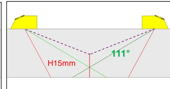
Almost no effect of the notch aperture as expected ( $\theta < 130^\circ$ )
