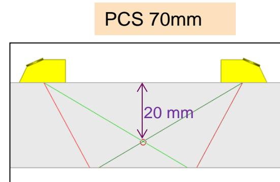
The amplitude of this reference simulated with CIVA (SOV model) is reliable (experimental validation study, L direct echoes of SDHs responses obtained for TOFD inspection, ICNDE 2012)
