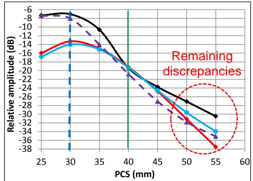
Effect of the notch aperture on the L diffraction echo of the top edge for incident angles > 130°
