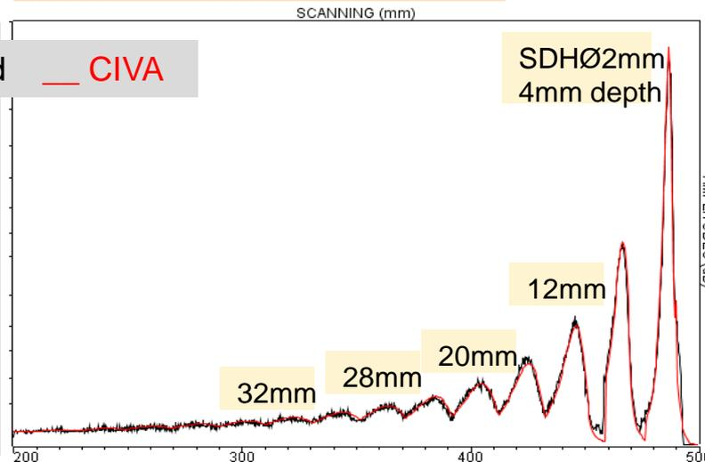
Measured and simulated SDH responses of each probe are very close:
