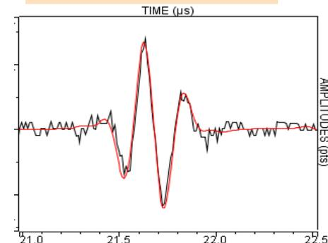
CIVA input signal parameters well adjusted by matching the experimental and CIVA Ascans
