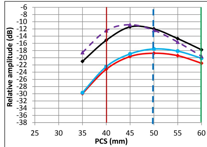
When taken into account the notch aperture effect, a good agreement for the amplitudes (and Ascans) between measure and CIVA-ATHENA 2D predictions
