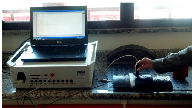
**FIGURE 4.** Ultrasonic pulse-echo apparatus.
