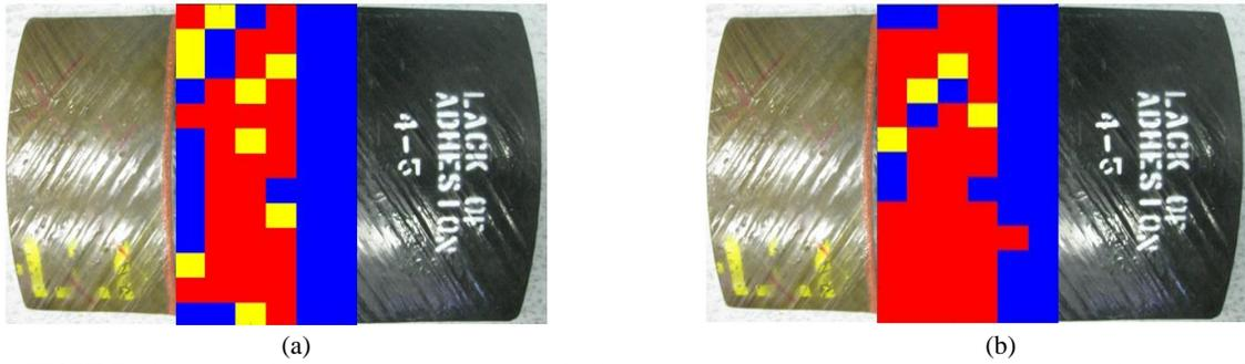
FIGURE 10. C-scans from specimens with lack of adhesion: (a) Lack of Adhesion 4-2 and (b) Lack of Adhesion 4-3
