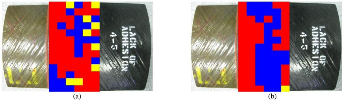
FIGURE 11. C-scans from specimens with lack of adhesive: (a) Lack of Adhesive 8-2 and (b) Lack of Adhesive 8-3
