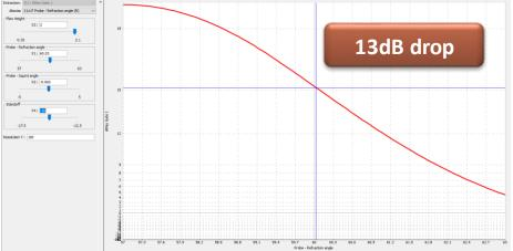
Refraction angle variation from 57° to 63° for a flaw height of 2mm, probe squint of -2° and probe standoff of 60mm.
