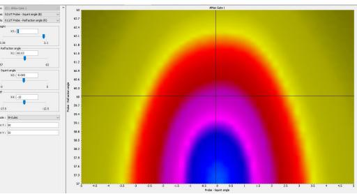
Refraction angle variation from 57° to 63° and squint angle variation from -5° to +5° for a flaw height of 2mm, and probe standoff of 60mm.
