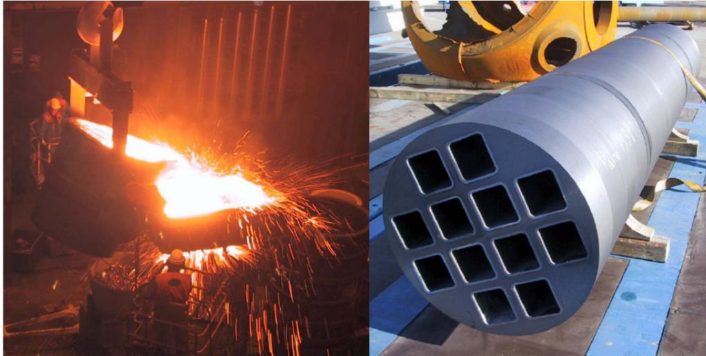
Figure 1 - Casting of nodular cast iron insert (left) and finally machined cast iron insert (right)
