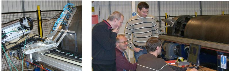
Figure 8 - Inspection of calibration block in the minirotorator on the left and both rotator and minirotorator are shown on the right.
