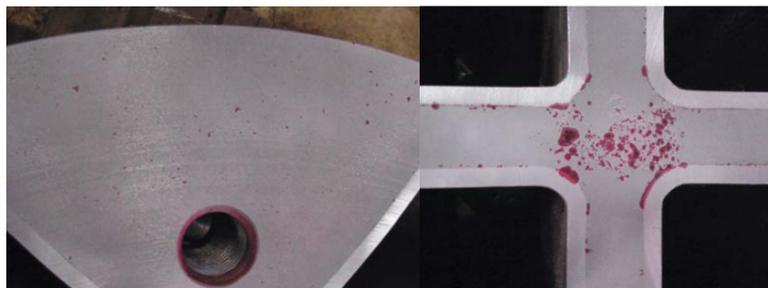
Figure 4 - Blowhole defects in the cast iron insert
