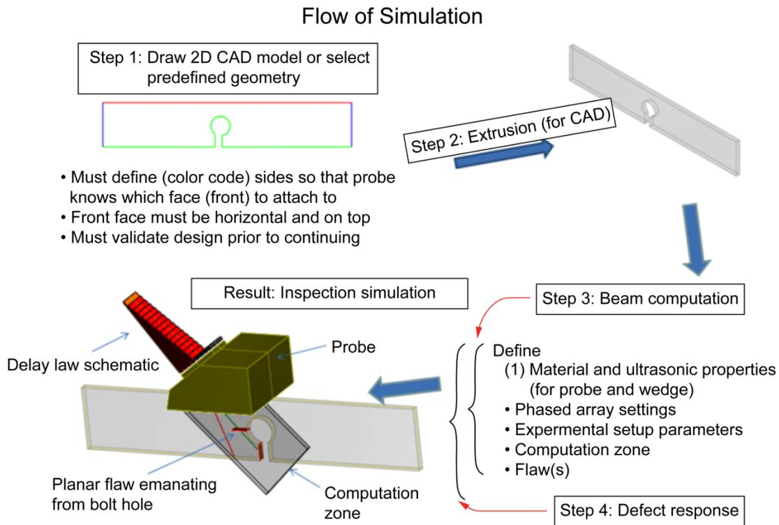
Simulation steps: (1) Two-dimensional profile of the isogrid test sample is drawn in the CIVA CAD facility. (2) The profile is extruded to create a three-dimensional solid model. (3) The material, setup, and flaw parameters are defined to create the inspection simulation. Beam computation can proceed after extrusion. (4) Defect response can proceed after flaw(s) is defined and inserted into the structure.
