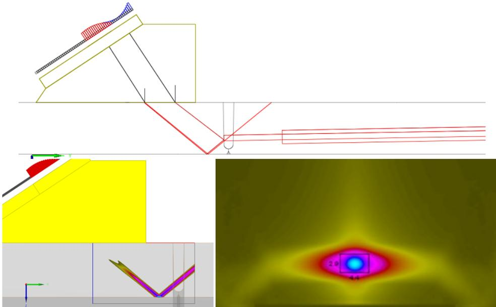
Figure 5: F2U channel views: a) Ray tracing, b) Transmitted beam calculated in the incident plane, c) spot sizing in the weld plane (2.9mm\*4.4mm at -6dB)
