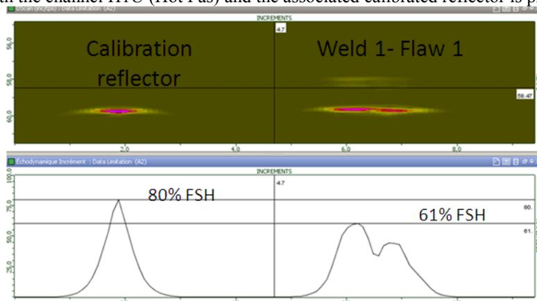
Figure 8: Simulated CIVA D-Scan and echodynamic charts for Weld1-Flaw1 with Channel H1U
