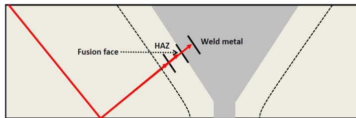
Figure 2: Acquisition gate adapted to fusion line region inspection
