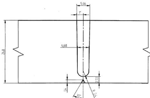
Figure 3: 1° J-Bevel weld cross-section
