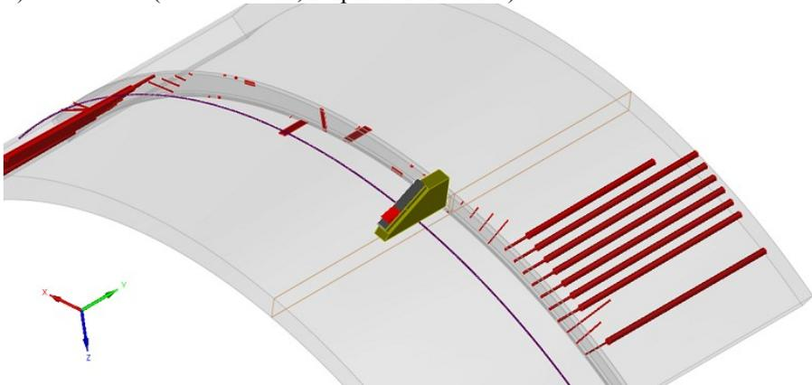
Figure 4: View of the calibration mock-up model in CIVA
