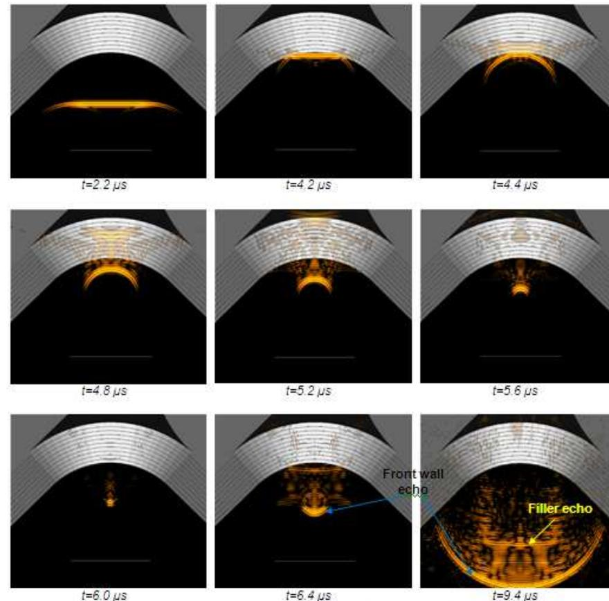
Figure 15 – Snapshots of ultrasonic propagation for the shot at 0° in log scale with 30 dB dynamic range
