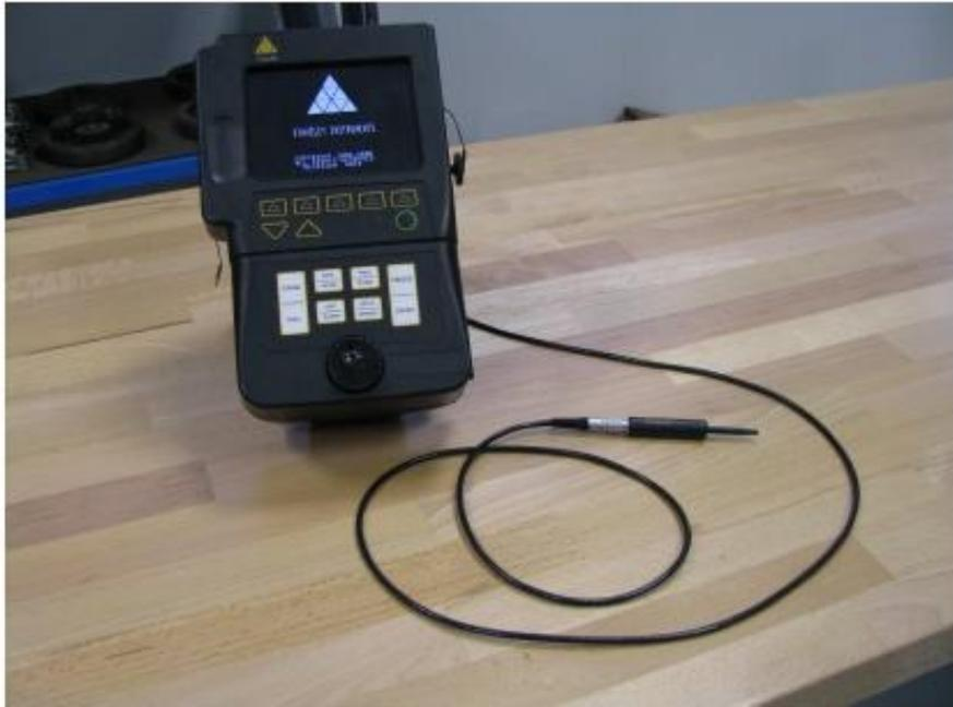
The calibration of the working frequency was carried out using an artificial known defect located on a specimen made of A1N
