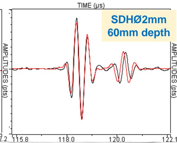
**Gaps in dB between the measured and the CIVA10.0 simulated maximal amplitudes**
