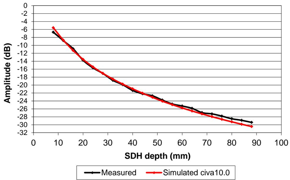
Immersion probe Ø12.7mm, 2.25MHz, SV45°, water path 50mm
