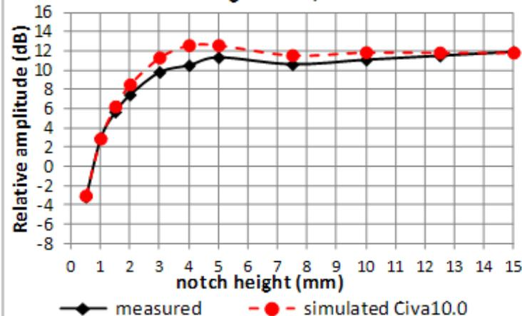
Immersion probe Ø6.35mm, 2.25MHz
