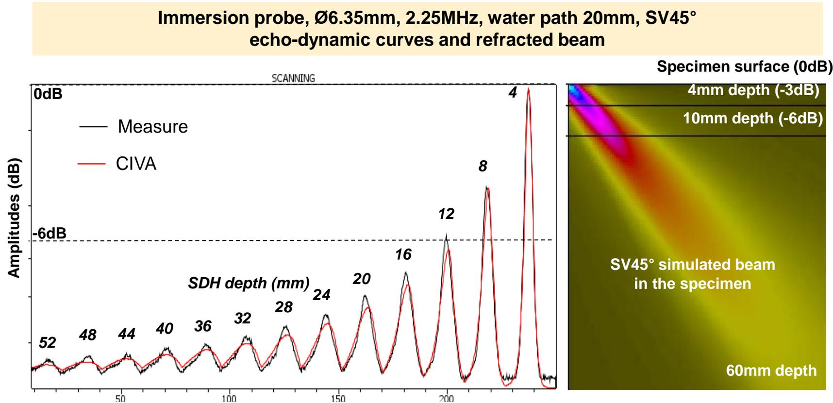
Small differences observed between simulation and measure both in amplitude and echodynamic curves shapes for deep SDHs
