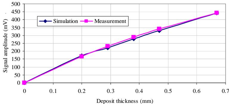
Simulation model validation vs experimental results (50% magnetite)
