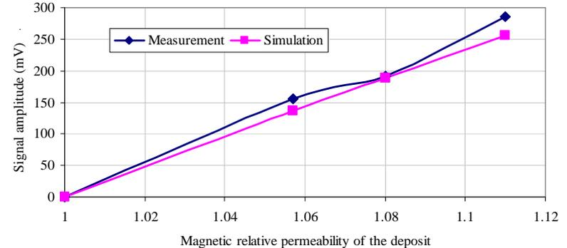
Relative permeability analytic formula validation vs correlation modelling/experimental results (0.23mm deposit)
