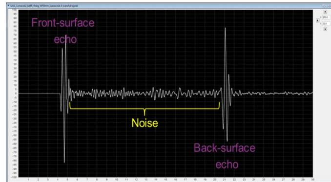
Presence of structural noise due to intermediate epoxy layers
