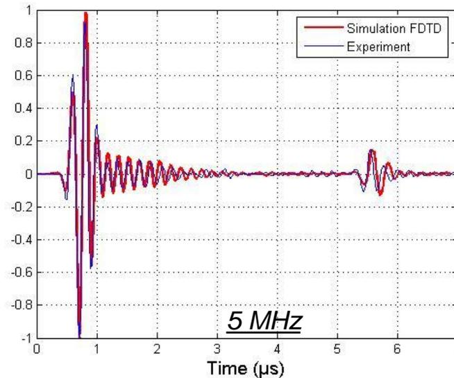
The amplitude of the backwall echo and the structural noise is well predicted by the model
