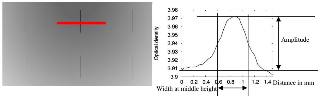
**Fig. 6.** Example of optical density profile extraction along the red line.
