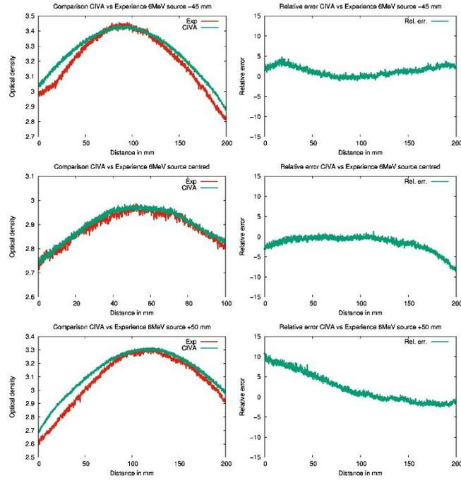
**Fig. 5.** Horizontal optical density profile along the notches mock-up: comparison between CIVA simulation and experimental data for 6 MV linear accelerator.
