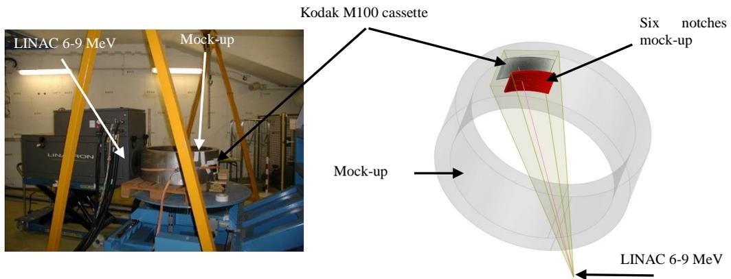
**Fig. 1.** On the left, real set-up. On the right, simulation set-up with CIVA RT.
