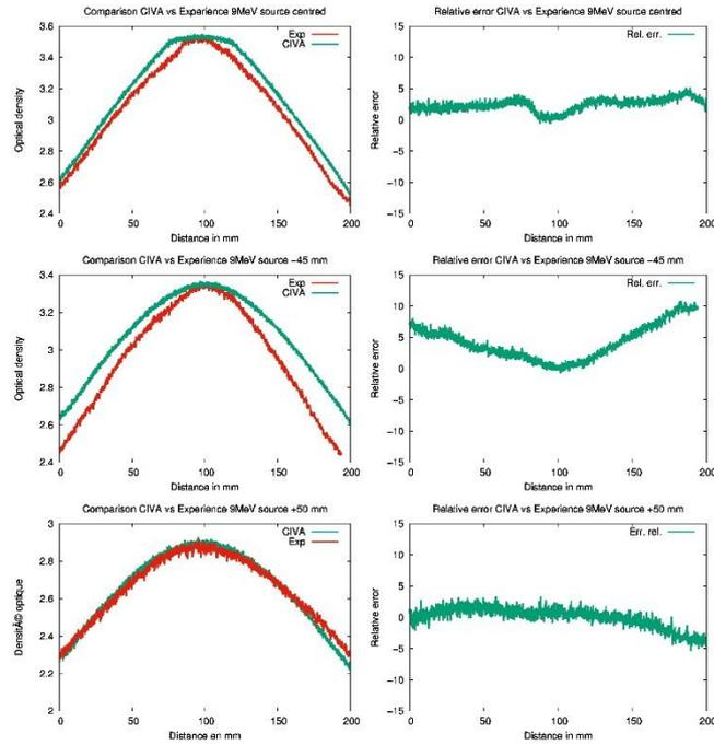
**Fig. 6.** Horizontal optical density profile along the notches mock-up: comparison between CIVA simulation and experimental data for 9 MV linear accelerator.
