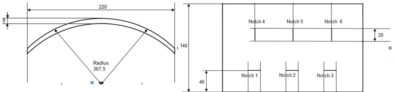
**Fig. 2.** Schema of the insert with the 6 notches.
