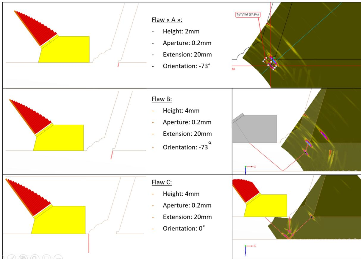
**Figure 13:** Simulated Defect scenarios and obtained sector scans
