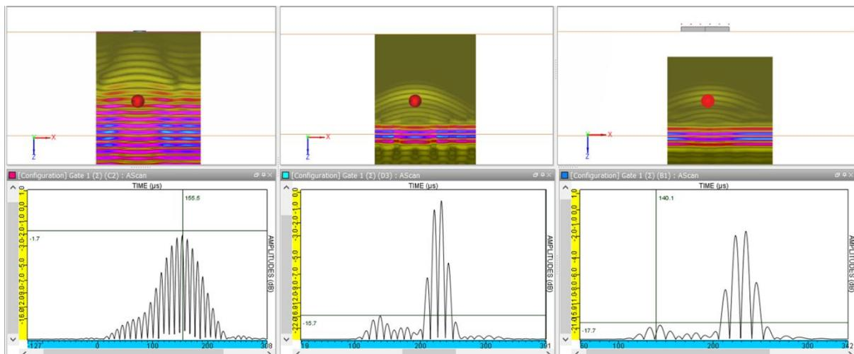
**Figure 3:** B-Scan images (at the top) and A-Scan signals when probe above defect location (at the bottom) for 3 ultrasonic transducers (from left to right: L0° probe, S1802, PL200 shear waves 0°)
