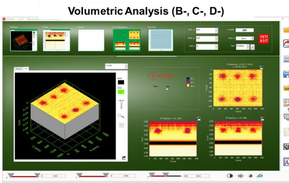
**Figure 5:** CIV4 simulation data exported in Echolyst analysis software.
