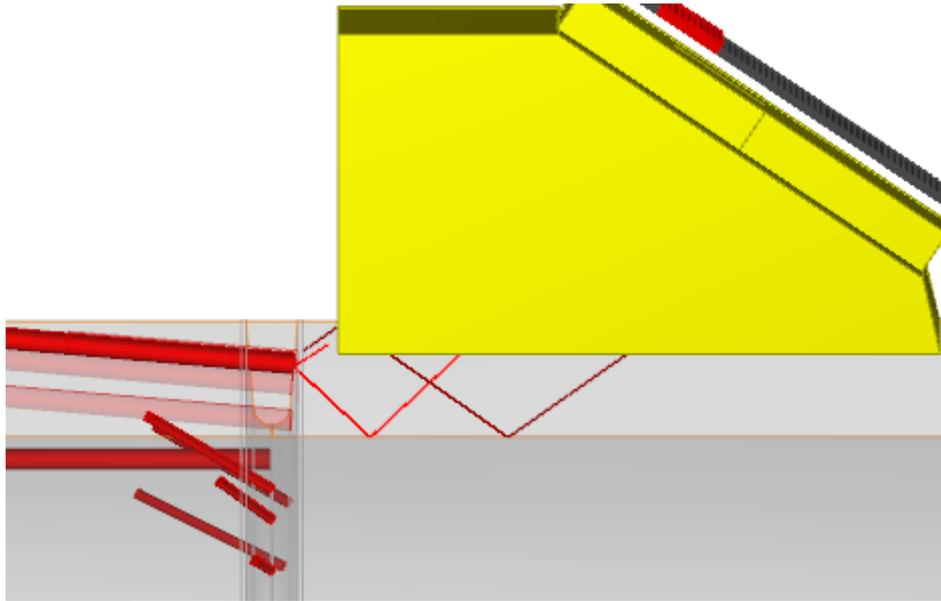
**Figure 4 Tx-Rx tandem ray paths for Fill 3 set to intersect on calibration targets**
