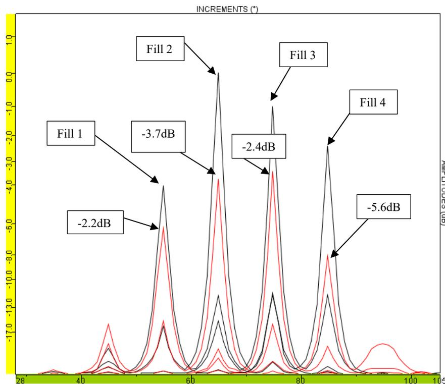
**Figure 9** Comparing echo-dynamics in fills. 2mm FBH (red) and 3mm FBH (black)
