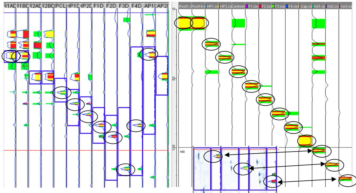
**Figure 5 Strip-chart validation scan of calibration block (PWZ left CIVA right)**
