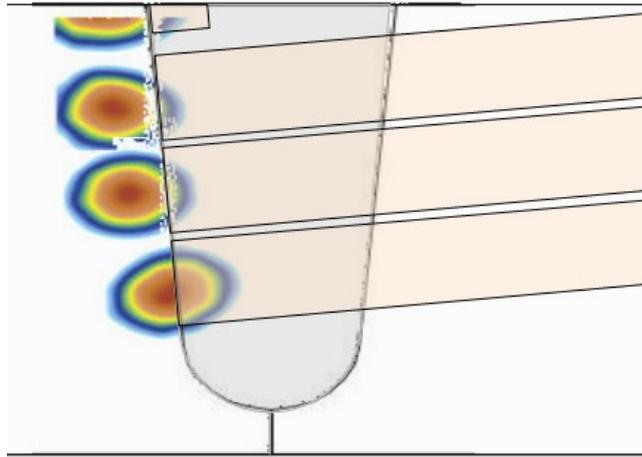
Figure 8 Sensitivity Coverage in 3 Fill Zones equalised including cap
