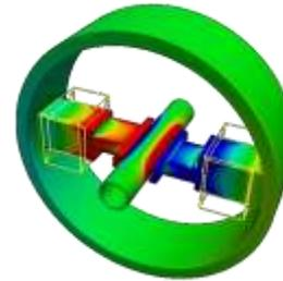
Oil & Gas applications: UT simulation of HTHA damaged specimen using UT advanced techniques : semi analytical Models of current CIVA version
