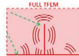
2. FEM computation of the diffraction inside the FE-Grid area + PML boundary conditions at box edges (i.e., no reflections)
