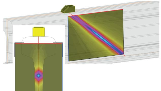
Beam computation in a rail component.
