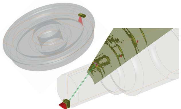
CAD files imported into CIVA. Wheel including a conventional UT probe and wheelset including a phased array probe.
