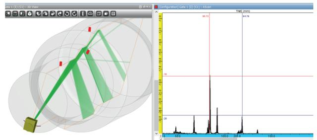
Rotating probe from the axle end. The three defects simulated will help estimate sensitivity for different defect locations and/or sizes.
