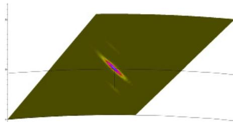
Same crack tilted -15° - height of 4 mm
