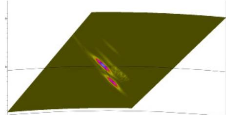
The defect orientation has a significant impact on the inspection result. The simulations visualize the signature of the defect as a function of orientation, greatly easing interpretation.
