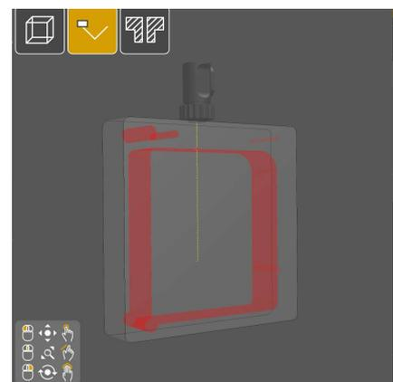
**Indications marking** and measurement tools mimic inspector practices. Setting up the **zone coverage** exercise is easy. Other features of the device have been enriched (signal auto set-up at 80% screen height, more gates available, several signal display options available, etc.).
