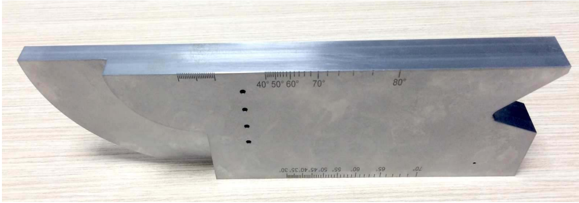
Fig. 6: The new PAUT block machined in accordance with ISO 19675
